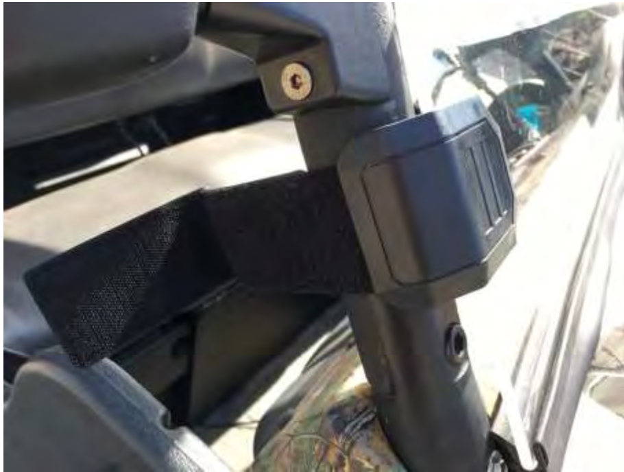
Install the windshield strap. Insert for the front.
